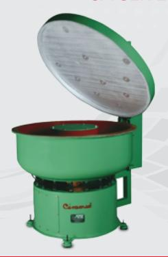
Vibratory machines use the principle of centrifugal force to cause vibrations to the work bowl thereby processing the components to the desired finish. The equipment comprises of a work bowl mounted on a rigid base frame.
